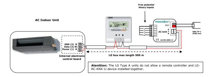
IntesisBox<sup>®</sup> LG-RC-KNX-1i allows monitoring and control, fully bi-directionally, all the functioning parameters of LG Air Conditioners from KNX installations. Compatible with VRF models commercialized by LG (see link to compatible models at the end of this document).
